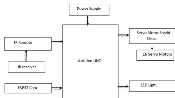
Fig7: Block Diagram
