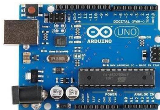
Fig1: Arduino UNO Board
